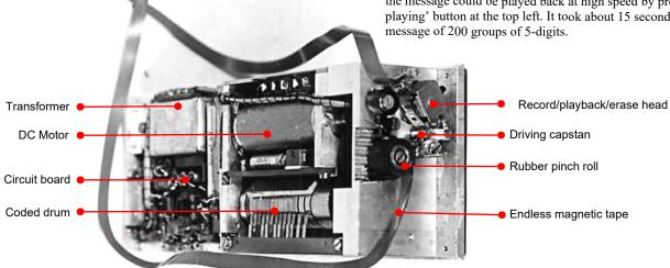
Bottom view of Dávač high speed Morse keyer. At the top centre was a DC motor which drove the coded drum and the recorder. Below was a coded drum comprising 10 notched rings, each of which represented a numerical character in Morse code. At the right was the recorder assembly which could be accessed from the side of the unit. It comprised an endless magnetic tape held in a small compartment, a rubber pinch roll, driving capstan, two tape guide capstans and record/playback/erase head.
