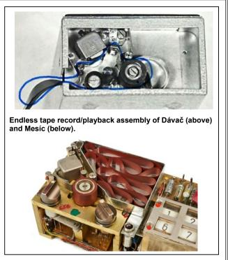
The operating procedure, general principle of operation and electronic circuit of the Dávač and Mesíc high speed Morse keyers was similar though its construction differed considerably. The main differences are tabulated below:
