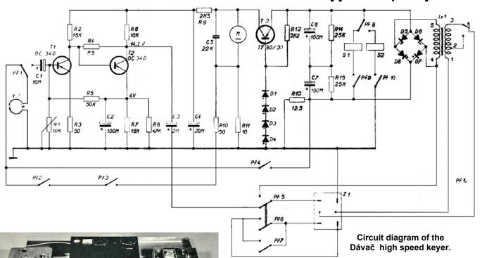
Photo left: Dávač high speed keyer connected to a Sirius I transmitter (centre top) via the rectangular 6-pin socket at the right hand side. On the left a Pluto receiver and a spares box to the right.
